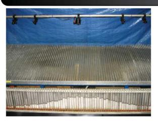
Flat Fan Spray with Tapered Edge and Wide Angle Allowing Uniform Spray Distribution Along Spray Boom at Various Spray Height.
